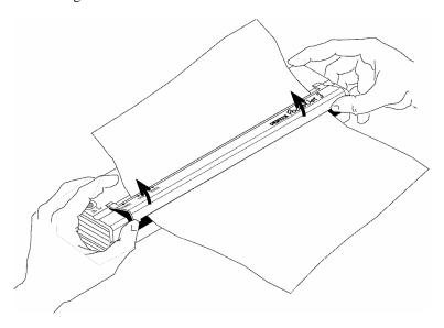
FIGURE 15. Opening the release cover
